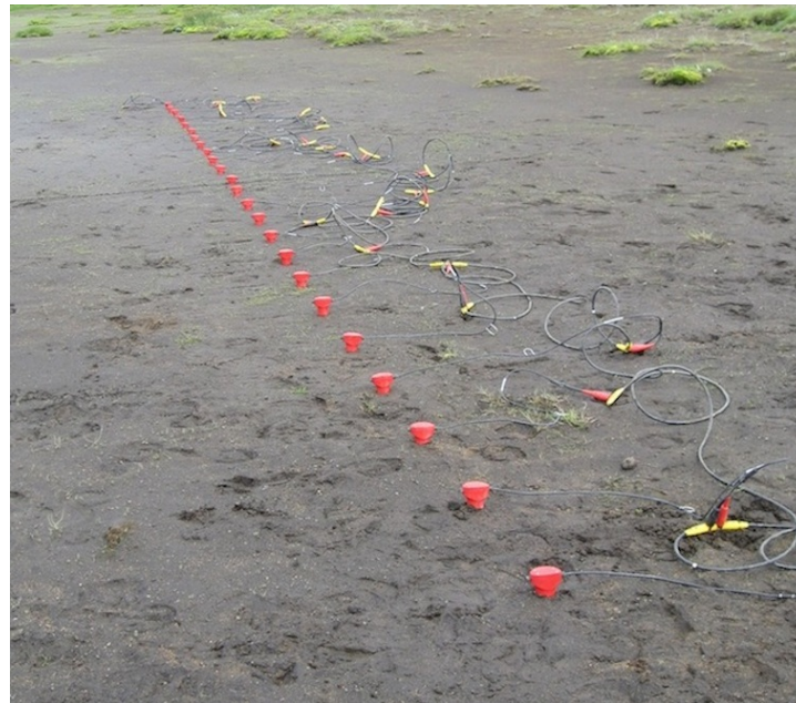
Figure 8.4: Typical MASW measurement profile. Line-up of 24 geophones with equal spacing.
