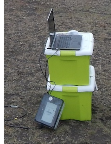
Figure 8.3: Data acquisition cards connected to a laptop computer.
